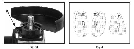
3. Seat the guard on the mounting flange. Rotate the guard to a position that will place the guard between the operator and the grinding wheel (or any other accessory requiring a guard). Tighten the clamp screw (A) Fig. 3A to secure the guard in proper position (see Fig. 4).
